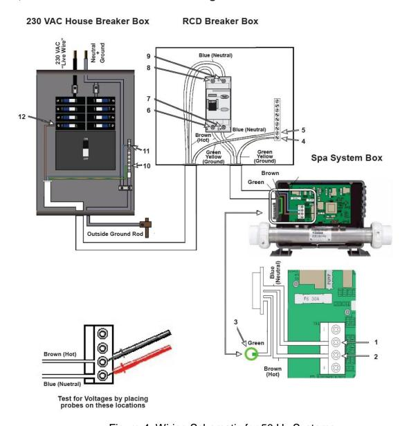
Figure 4. Wiring Schematic for 50 Hz Systems
