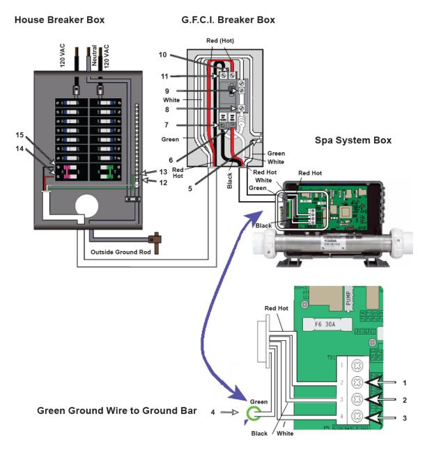
Figure 2. GFCI Wiring Schematic for 60 Hz Systems
