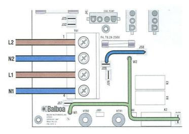
Figure 6. Two Phase Power – TN and TT Electrical Systems 2 x 16 A, 5 Wires (2 Lines + 2 Neutrals + 1 Protective Earth)
