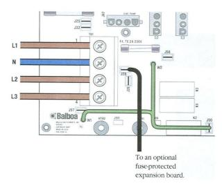
Figure 7. Three Phase Power – TN and TT Electrical Systems 3 x 16 A, 5 Wires (3 Lines + 1 Neutral + 1 Protective Earth)
