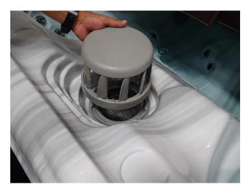
Figure 14. Weir cap removal
