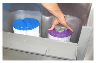
Figure 18. Screw-in Filter Removal
