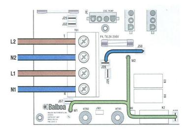
Figure 5. Two Phase Power – TN and TT Electrical Systems 2 x 16 A, 5 Wires (2 Lines + 2 Neutrals + 1 Protective Earth)
