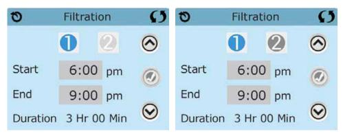
Press "1" to view Filter 1. Press "2" once to view Filter 2. Press "2" again to turn Filter 2 ON or OFF.
