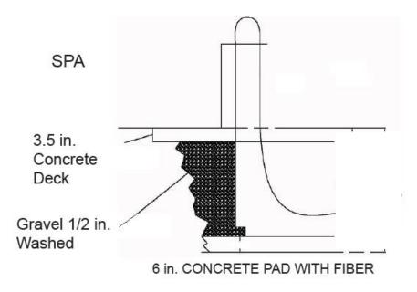
Figure 9. Excavation Cross Section
