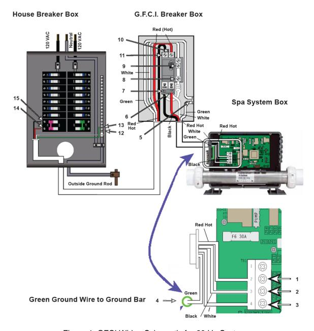
Figure 1. GFCI Wiring Schematic for 60 Hz Systems
