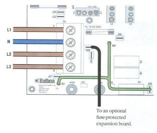
Figure 6. Three Phase Power – TN and TT Electrical Systems 3 x 16 A, 5 Wires (3 Lines + 1 Neutral + 1 Protective Earth)
