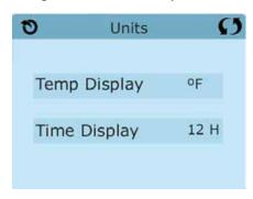
Press "Temp Display" to change the temperature between Fahrenheit and Celsius.
