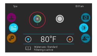
When done adjusting the speed of the swim pumps, the screen will return to the main screen. The WaVS pump button will now be illuminated in color to incicate that the swim pumps are on.
