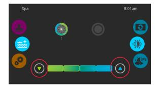
By pressing the up/down arrows on either side of the speed bar will adjust your swim pump speeds in that direction in small increments.
